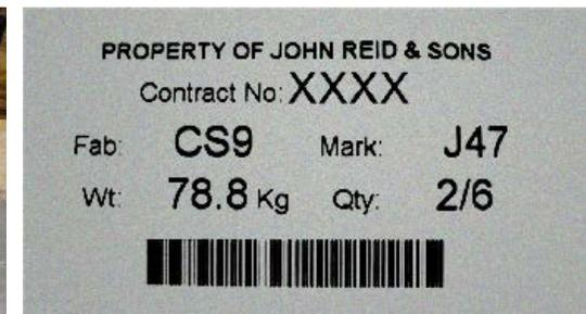
■ Packing labels show the contract number, fabrication issue, assembly mark number, weight and the item number/quantity - in this example above it is denoting item 2 from a total of 6.
