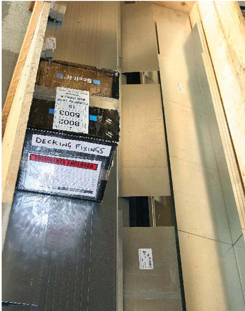
■ Every steel piece is identified by a 'Mark Number' and has a label showing this and other production information. We have a comprehensive system of listing and checks so each piece can be accounted for in accordance with our ISO 9001 system and European CE Mark compliance.
